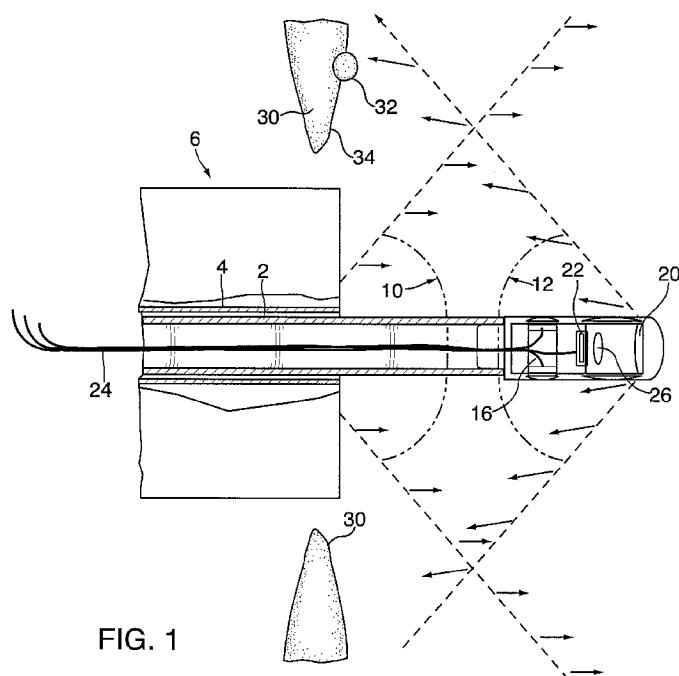
(57) Abstract: An endoscopic imaging catheter is configured for insertion, optionally via a longitudinal channel of an endoscopic insertion tube. The endoscopic imaging catheter includes reflecting and optical elements and an imaging element. The reflecting element reflects onto the imaging element through the optical element side and rear views of at least a portion, or the entire 360° view of a wall encircling an intrabody lumen around the axis of said the longitudinal channel.
