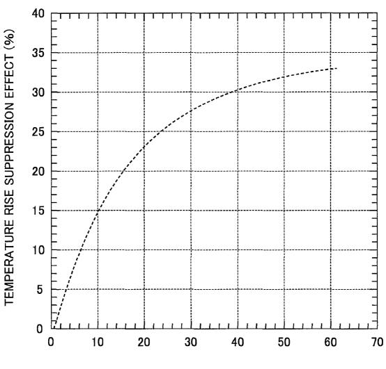
COEFFICIENT OF THERMAL CONDUCTIVITY OF EXTERIOR MEMBER (W/mK)
