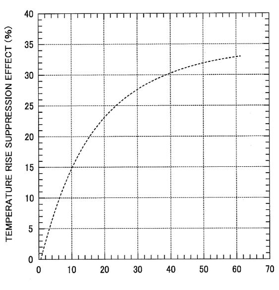
COEFFICIENT OF THERMAL CONDUCTIVITY OF EXTERIOR MEMBER (W/mK)
