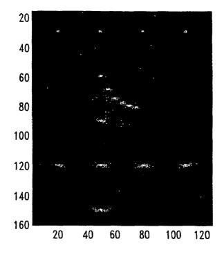
SPATIALLY COMPOUNDED IMAGE RECONSTRUCTION USING UNIFORM ILLUMINATION METHOD. FIVE FLAT WAVEFRONT PULSES WERE USED AT STEERING ANGLES OF -20, -10, 0, 10, AND 20 DEGREES. INTENSITY DATA ARE COMPRESSED WITH A SQUARE ROOT FUNCTION.
