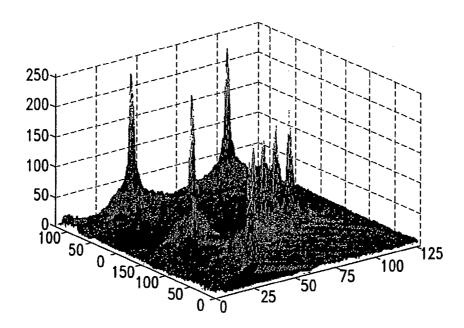
PERSPECTIVE VIEW OF ZOOMED REGION OF FIG. 6, WITH IMAGE POINTS AT 1/2 WAVELENGTH SPACING. PINK COLOR HIGHLIGHTS SIDE LOBES AT -48DB OR LOWER, WHILE DARK BLUE COLOR SHOWS BACKGROUND CLUTTER AT LESS THAN -100DB. SCALE ALONG X AND Y AXIS IS IN 1/2 WAVELENGTH UNITS.
