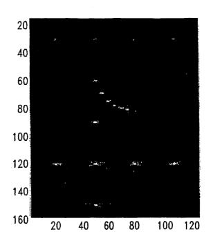
MATLAB SIMULATION OF PIXEL-ORIENTED PROCESSING METHOD. THE POINT TARGETS SHOW THE TYPICAL CROSS-SHAPED PATTERN FOR SLIDE LOBES (INTENSITY DATA ARE COMPRESSED USING A SQUARE-SHAPED PATTERN FOR SIDE LOBES (INTENSITY DATA ARE COMPRESSED USING A SQUARE ROOT FUNCTION). SCALE ALONG X AND Y AXIS IS IN WAVELENGTHS.
