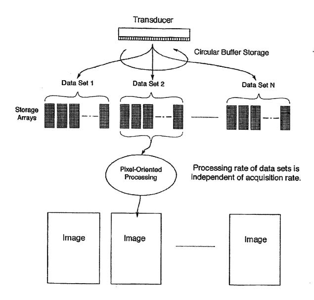
Processing of output image frames can be performed at different rate than acquisition rate.
