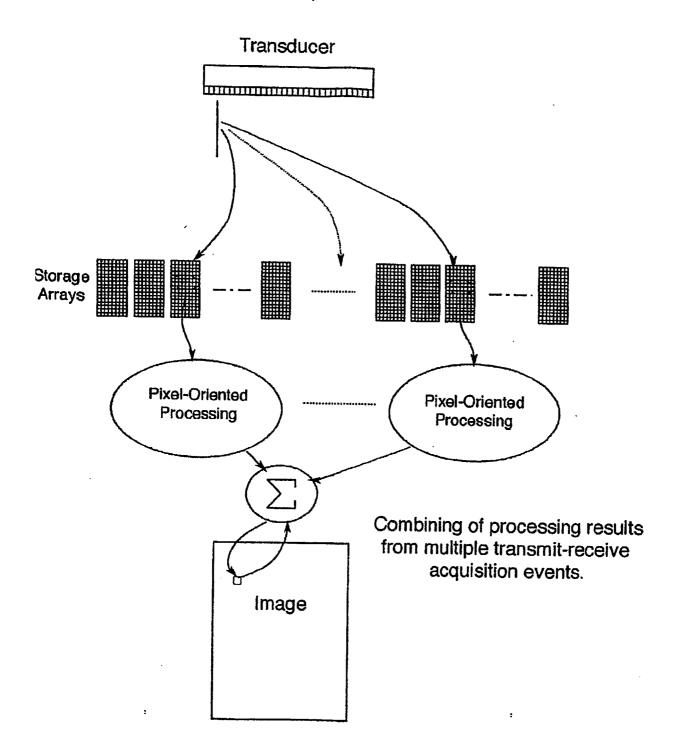
Processing results from multiple acquisitions can be combined to improve output pixel signal.
