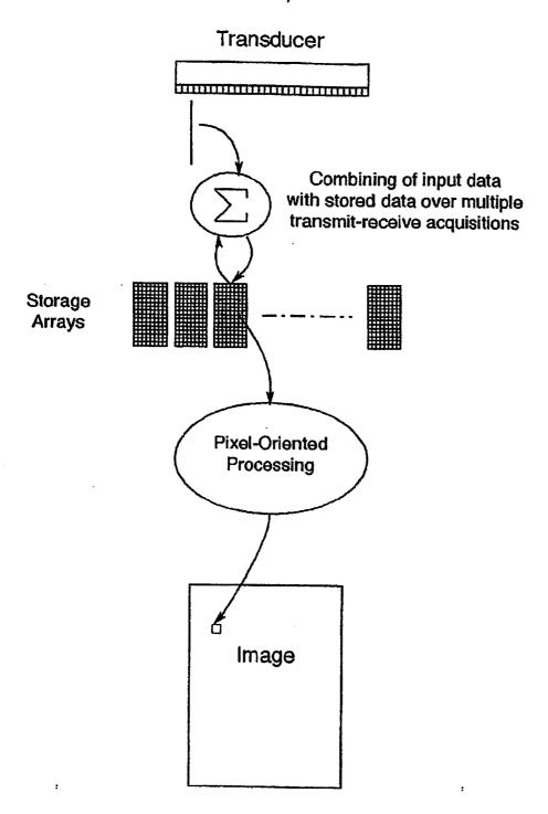
New acquisition data can be combined with data in storage to improve input signal quality.
