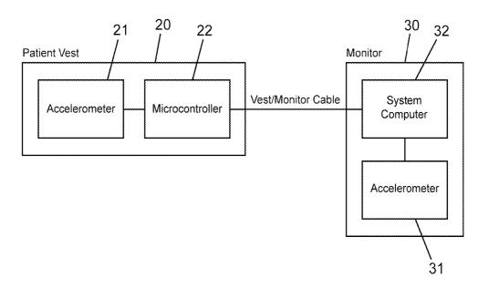
**Figure 3: Monitor Accelerometer**
