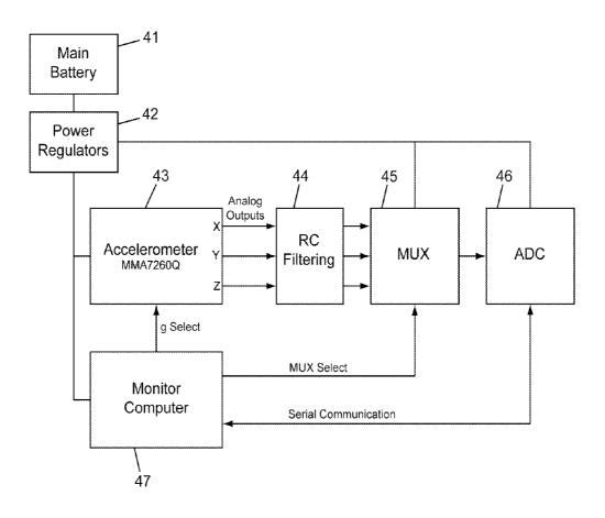
Figure 4: Belt Node Accelerometer
