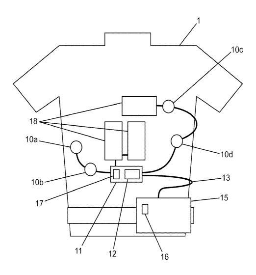
Figure 2: System diagram with accelerometers
