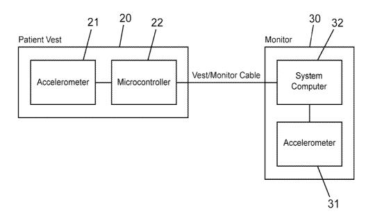
**Figure 3: Monitor Accelerometer**
