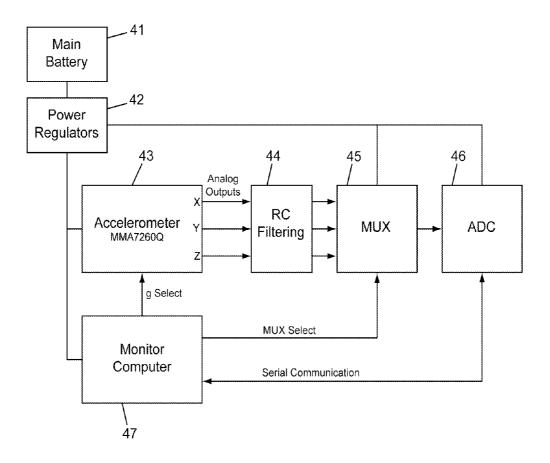
**Figure 4: Belt Node Accelerometer**
