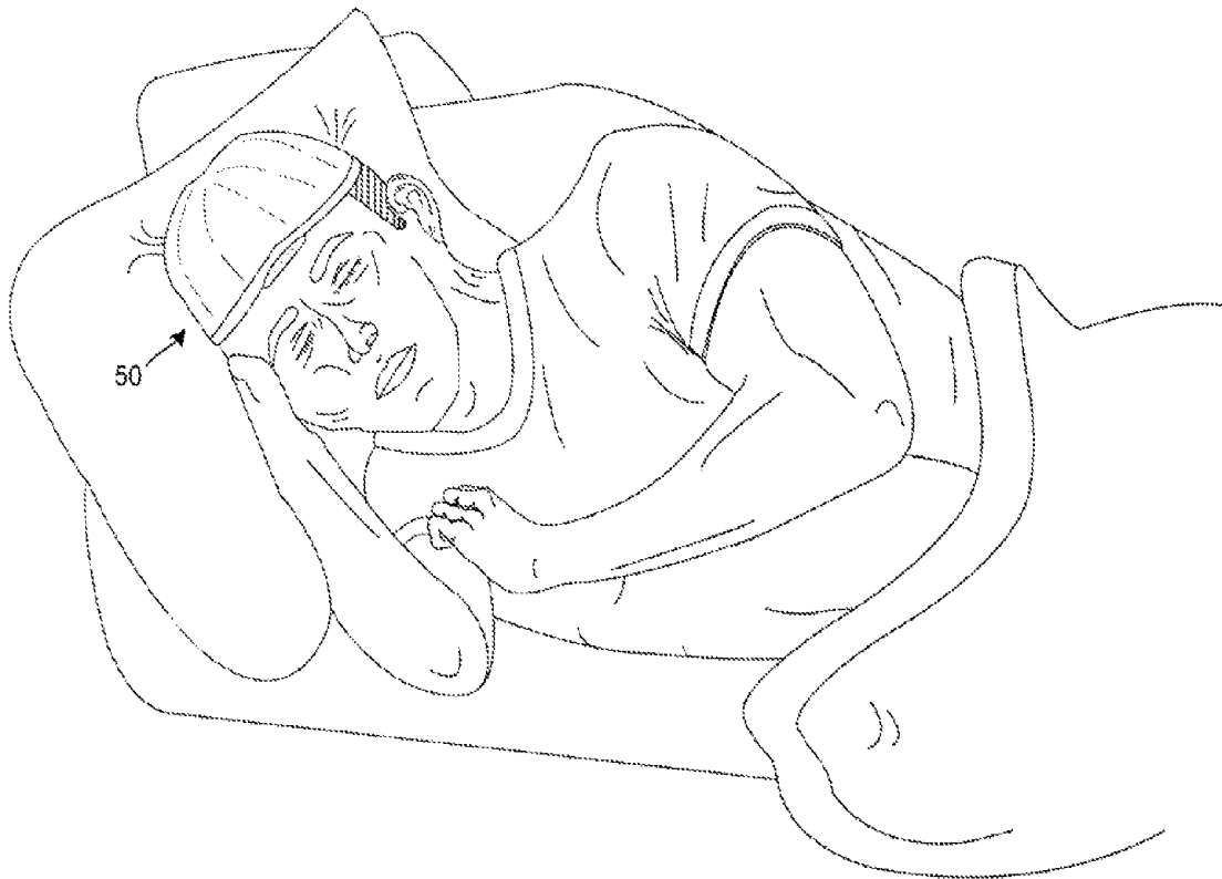
HEAD CAP SECURES SENSORS TO FOREHEAD DURING SLEEP
