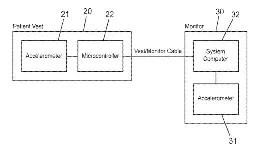
Figure 3: Monitor Accelerometer
