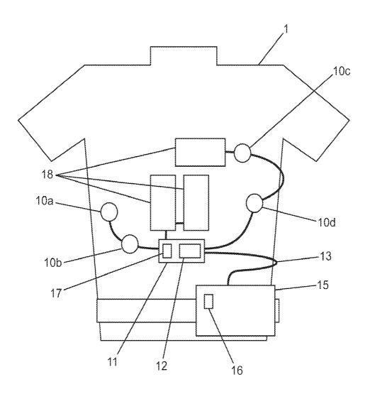
Figure 2: System diagram with accelerometers
