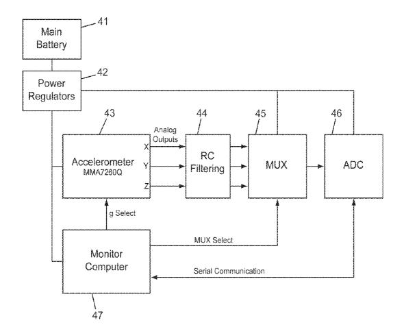
Figure 4: Belt Node Accelerometer
