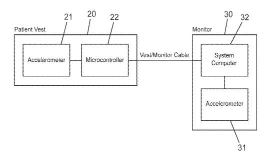
Figure 3: Monitor Accelerometer
