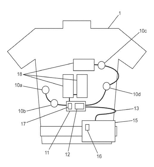
Figure 2: System diagram with accelerometers
