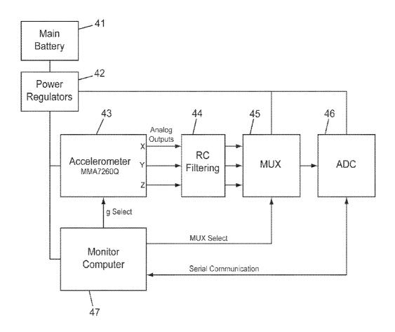
Figure 4: Belt Node Accelerometer
