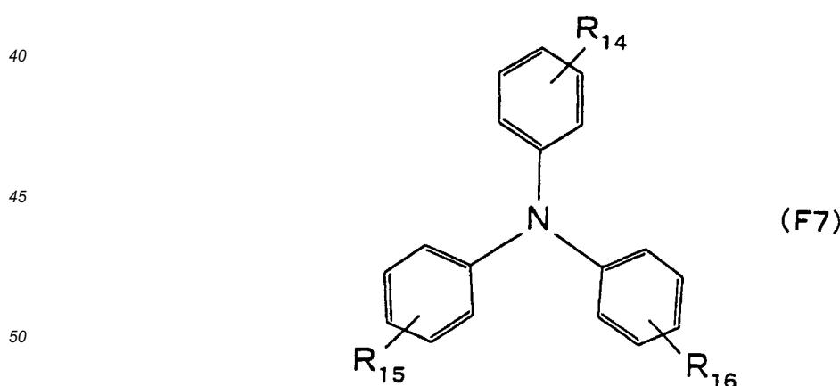
wherein at least one of R13, R14 and R15 is styryl, phenylstyryl, naphthylstyryl, or a derivative thereof substituted by an alkyl group, an amino group or a phenyl group; and R13, R14 and R15 other than the above are respectively made of an alkyl group, an amino group, phenyl group, alkyl-substituted benzene, or amino-substituted benzene.
