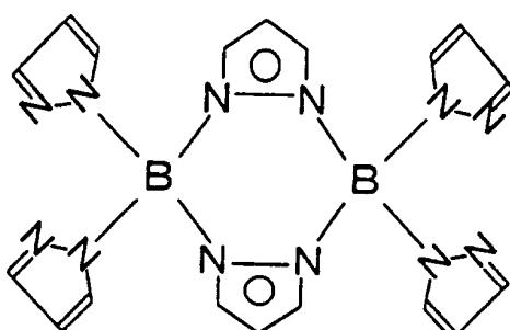
[0072] The above-mentioned organic material for an EL device is suitable for material of the light emitting layer of the EL device. Furthermore, since the above-mentioned organic material for the EL device is an electron-deficient compound, it is also suitable for the material for the electron transport layer or the electron injection layer of the EL device.
