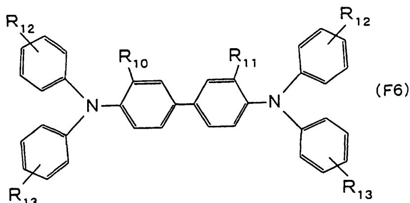
wherein R10 and R11, which can be same or different, respectively denote one selected from the group consisting of hydrogen, a methyl group, a methoxy group and Cl; and R12 and R13, which can be same or different, respectively denote one selected from the group consisting of hydrogen, an alkyl group, an alkoxy group, a phenyl group and a phenyl group substituted by an alkyl group or an alkoxy group.
